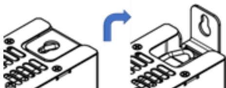
Figure 2 - Opening flip-flange for mounting plate fastening
